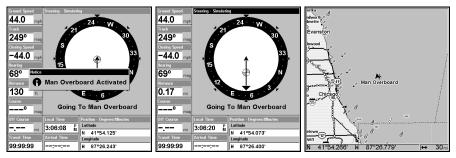
Navigating to Man Overboard: Man Overboard Activated message, left. Navigation Page, center, Map Page, right. The victim is to the starboard of the vessel. The GPS shows which direction to go for the rescue.
